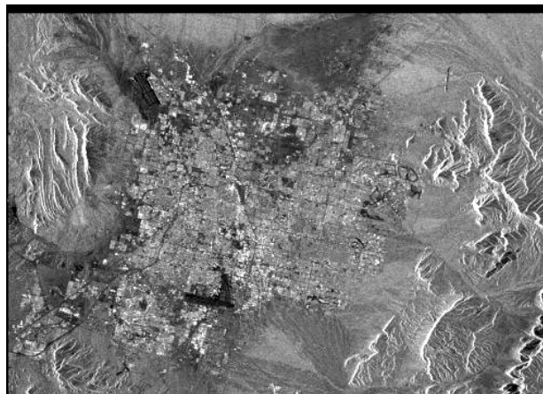
Figure B1. Multi-look intensity image 25394.mli (1800 pixels long and 2500 pixels wide, pixel size 20 m in ground range and azimuth direction).
